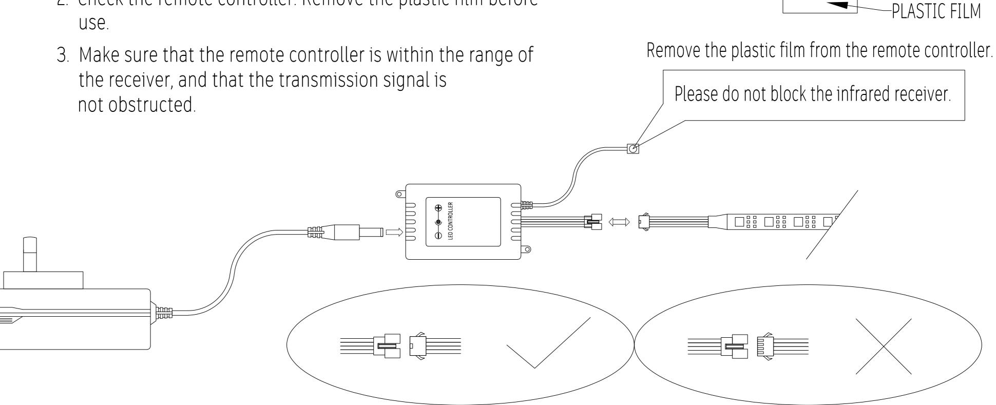
Check the facing of the connectors and ensure that they are aligned correctly.
