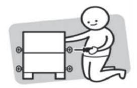
Do not fully tighten all screws until the step or process has been completed.
