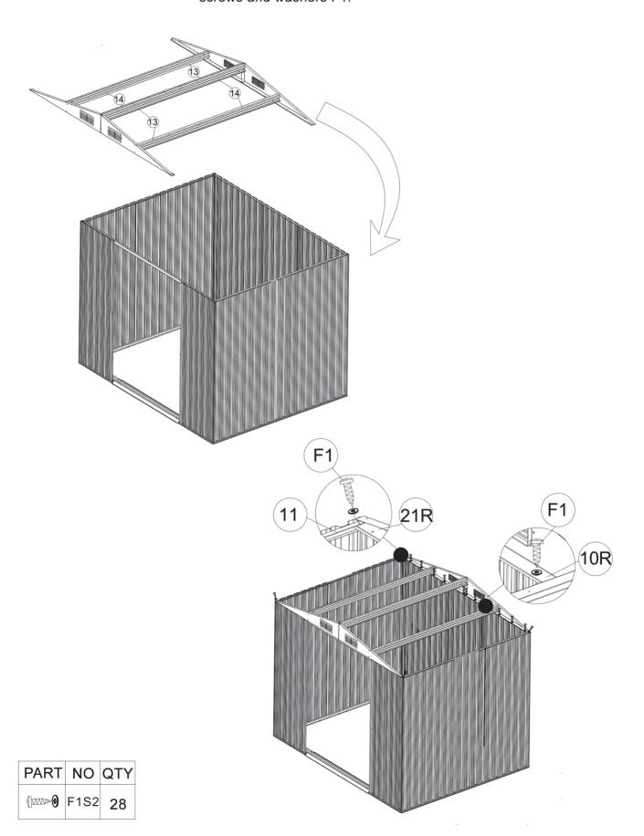
Place the roof panels (P5, P6 and P7) on top of the gable panels. Line up the holes and secure the assembly with screws and washers F1.
