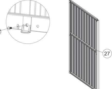
Attach two door handles (GB) to the door panels (D2) and secure them with nuts, bolts and washers F2.
