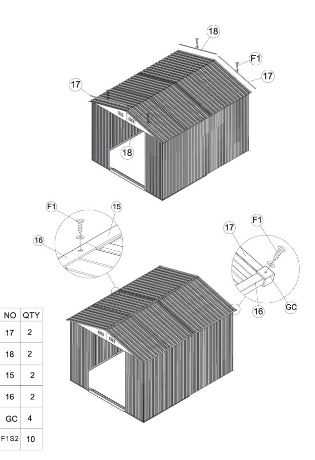
Attach two centre roof flashings (19) on top of the roof panels as shown. Secure them with screws and washers F1. Then attach the flashing end caps (GE) to both ends of the centre roof flashing and secure with screws and washers F1.
