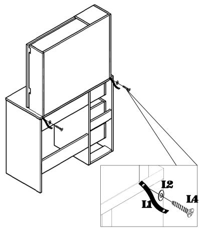
Attach **11** to back of cabinet with screw **14** and washer **12**.
