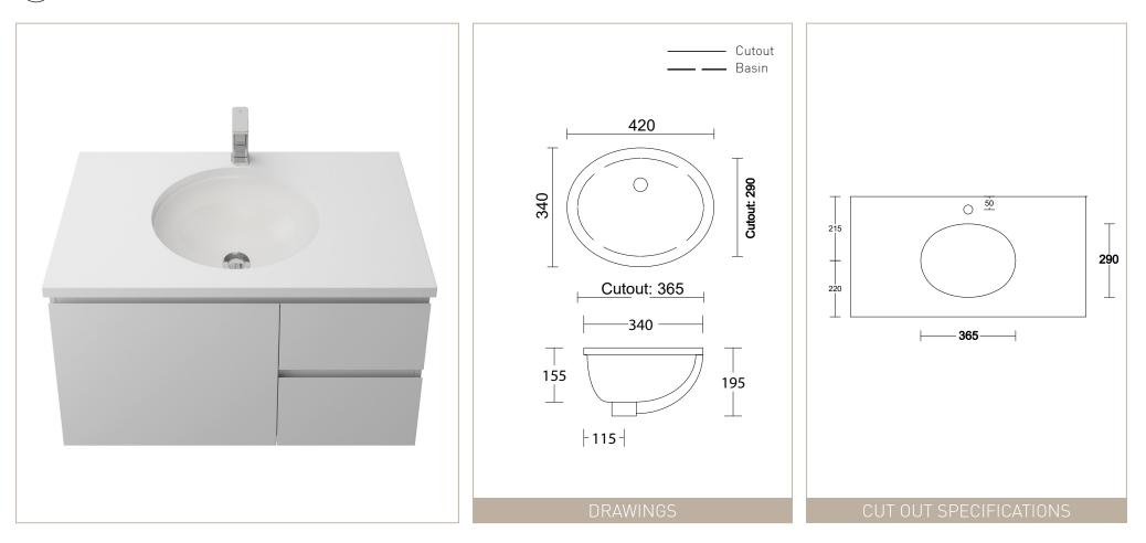
NOTE: Waste not included Waste Size: 32mm Overflow to: Front of Basin Minimum Depth: 460mm with taphole behind, 420mm without taphole behind
