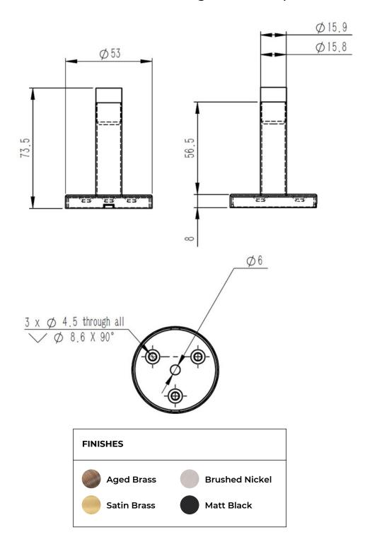
Fixings: Supplied with 3 x Timber Fixing screws and 3 x Masonry Plugs
