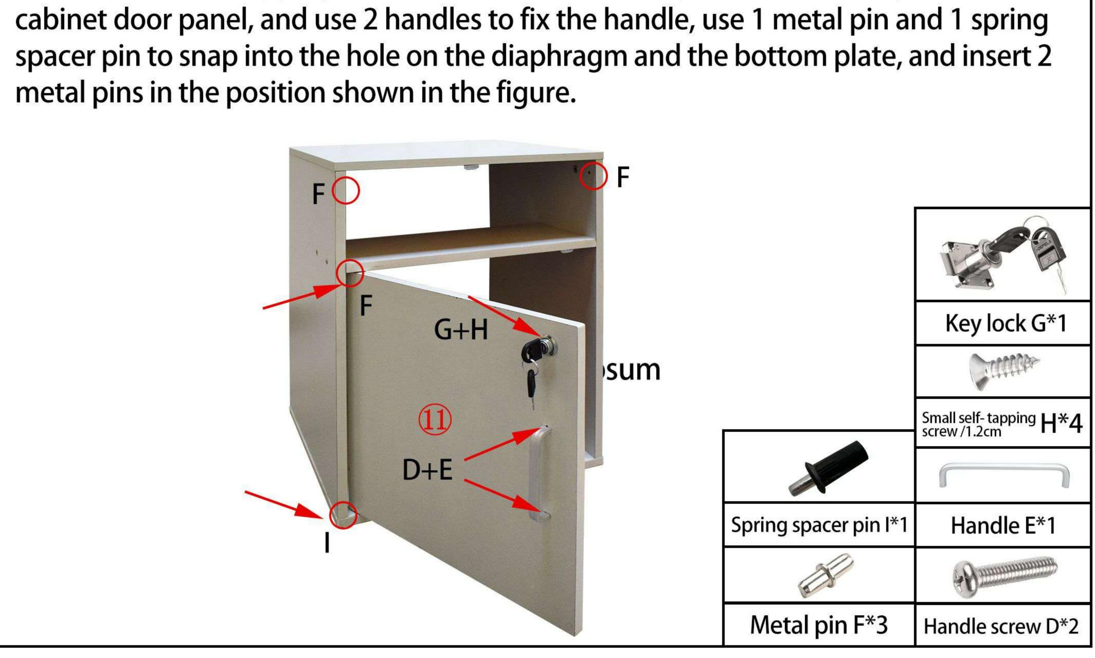
6. Use 4 small self-tapping screws on the cabinet door panel to fix the key lock on the
