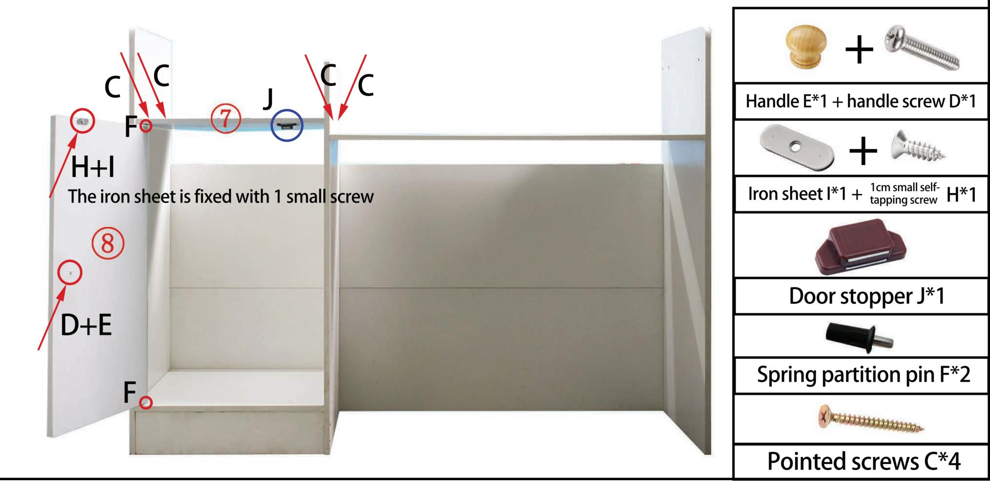
7. Align the hole position of the front upper baffle with the wooden tip position of the middle baffle and insert it, fix it with 4 pointed screws and the left and right vertical plates, and screw in 1 eccentric screw in the position shown in the figure.
