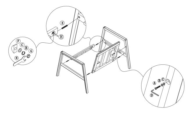
Step 2: Put the seat plate on the main connecting wood, by self-tapping locks from bottom to top (12 for hardware I, 1 for J)
