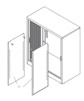
Fix H in the body with 4 screws
