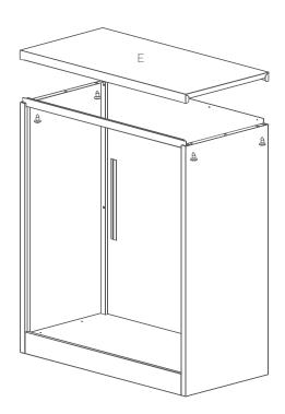
Fix E in the body with 6 screws
