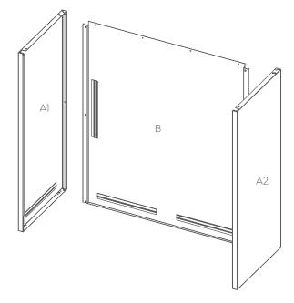
Link A1 & A2 with B and fixed by 6 screws.
