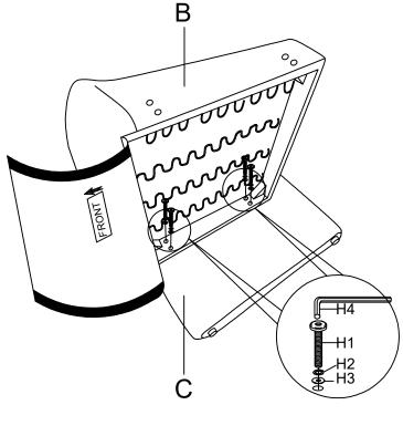
Put screws to holes to connect left arm & rightarm to seat, tighten to 60%
