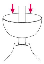
8. Place the hanging ball on top of the down rod and secure it with the ball pin and two screws. **CAUTION**: Secure one screw through holes on the hanging ball and the down rod.
