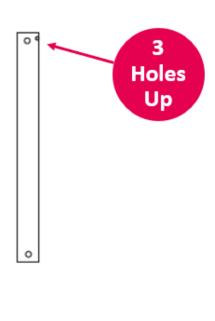
8. Feed the main motor wire plug and light wire plug (light version only) up through the inside of the downrod, then insert the downrod into the downrod holder. Gently push the cross-pin through the holes aligned with the base of the downrod holder and downrod.
