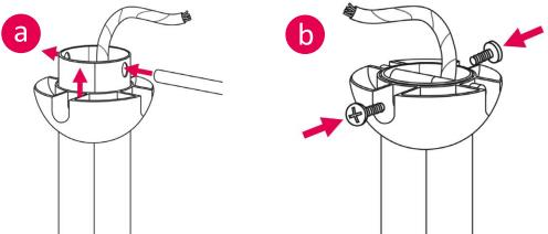
9. Hang the fan into hanging bracket. Align ball groove on hanging ball with ridge on hanging bracket. Ensure hanging ball sitting into hanging bracket correctly. If fan doesn't sit properly, hold the downrod and twist it until fan has been secured into hanging bracket.
