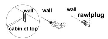
STEP 2: Insert screw through strap into hole in wall
