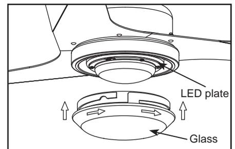
9. Secure the glass to LED plate by twisting in a clockwise direction. Do not over-tighten.
