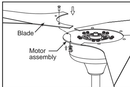
2. Reassemble the blades to the motor assembly using the previously removed screws, spring washers and hex nuts. Rehang the fan.
