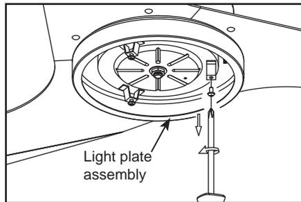
5. Remove one of the three screws in the light plate assembly and retain the removed screw for next step. Slightly loosen the remaining two screws.
