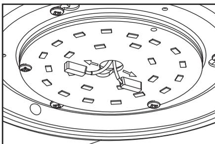
7. Push end of light wire into either connector on the LED plate. Repeat with other wire to other connector.
