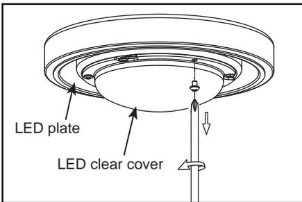
4. Disassemble the LED clear cover from the LED plate by removing three screws and retain the removed screws for Step 8.
