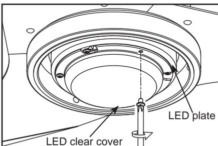
8. Reassemble the LED clear cover to LED plate using the previously removed screws.
