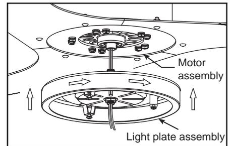
3. First pull out light wire lead and remove the shrinkable sleeve then through the hole in the light plate assembly. Assemble the light plate assembly to the motor assembly by twisting in a clockwise direction until tight.
