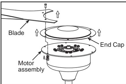
1. Remove the blades and end cap from the motor assembly. Retain the blades and screws, spring washers and hex nuts for next step.
