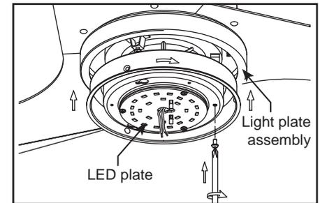
6. Assemble the LED plate to light plate assembly using the two key slots. Replace the third screw and securely tighten all three screws.
