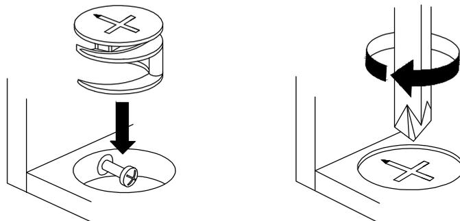
Turn cam lock clockwise to tighten.
