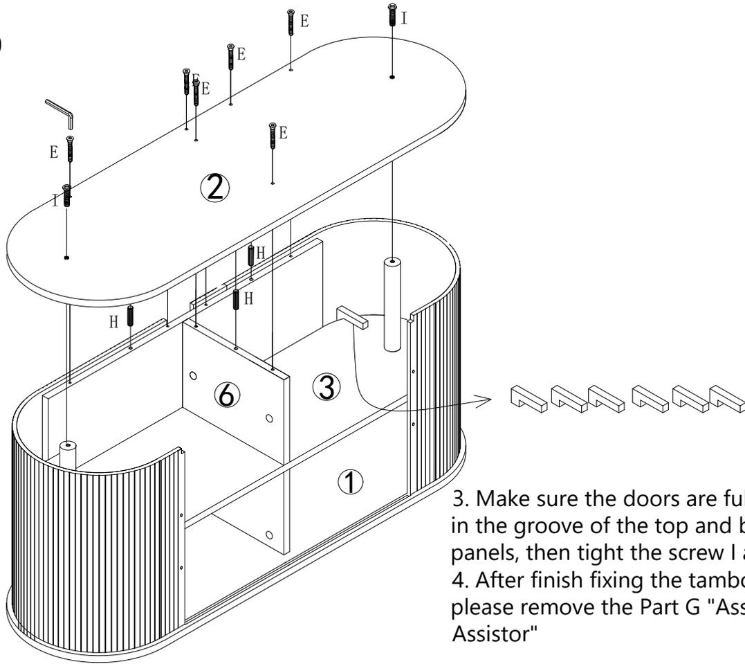
3. Make sure the doors are fully inserted in the groove of the top and bottom panels, then tight the screw I and E.
