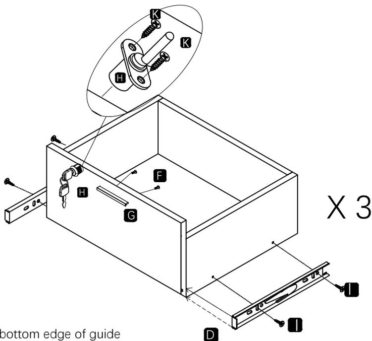
1. The bottom edge of guide rail should align at the bottom edge of the side board.
