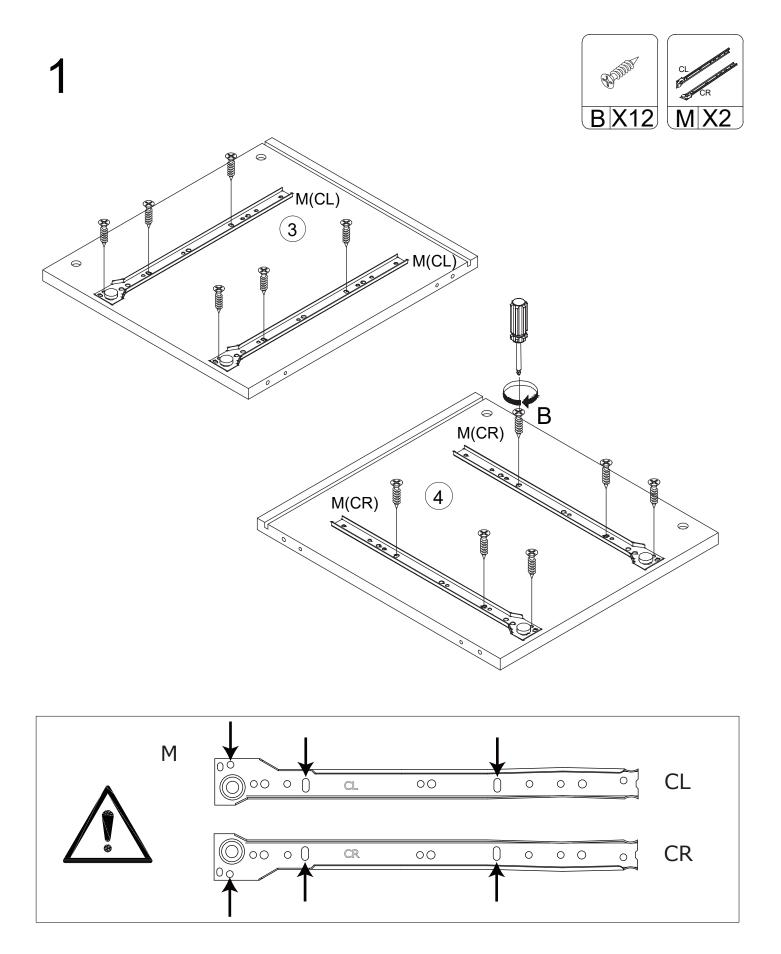
Fix 2 x Slide Tracks M (CL) onto Left side panel (3) with 6 x Screws (B) using a screwdriver. Fix 2 x Slide Track M (CR) onto Right side panel (4) with 6 x Screws (B) using a screwdriver.
