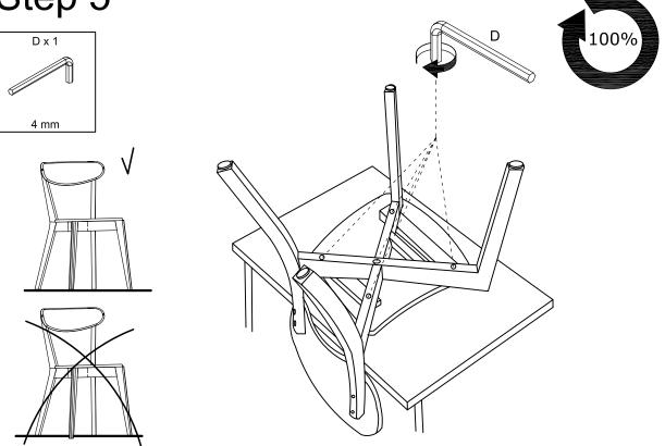
Tighten all Bolts 100% but do not over tighten
