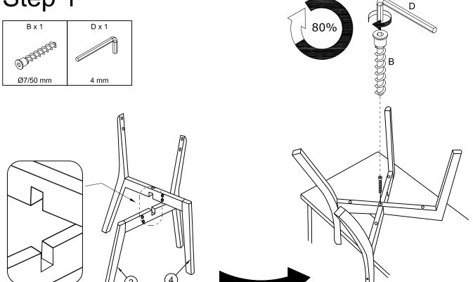
Screw the Bolt only 80% of the way and do not over tighten
