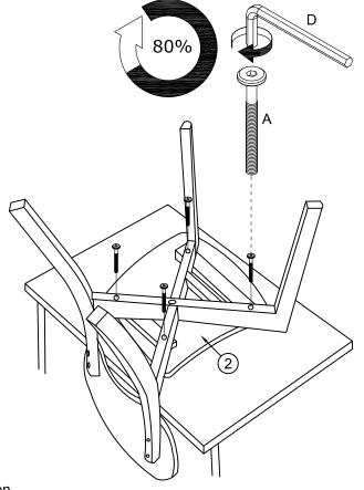
Screw the Bolts only 80% of the way and do not over tighten
