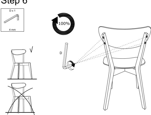
Tighten all Bolts 100% but do not over tighten
