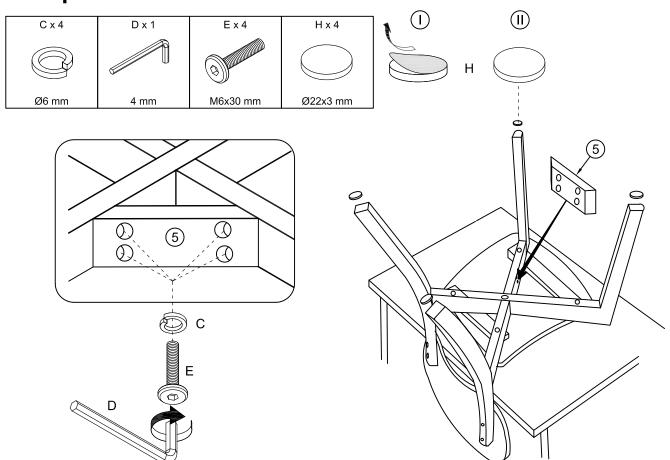
Tighten all Bolts 100% but do not over tighten Attach the Felt Pads to the Legs
