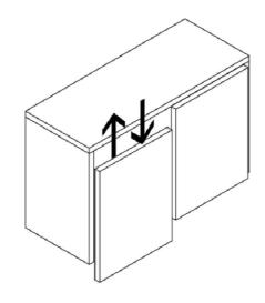
Vertical Adjustment via mounting plate (via slots or, if in two pieces, via screw)
