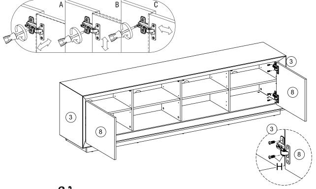
Attach 2x Door (8) to case assembly as shown. Adjust the Door hinge until fix.
