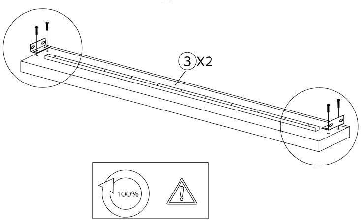
Attach 2x Sideboard(3) to Headboard(1) and Footboard (2) with Nuts have been installed.
