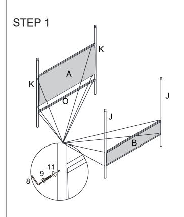
Note: Assembled one side first,Do not fully tighten the bolts until the other side tightening.
