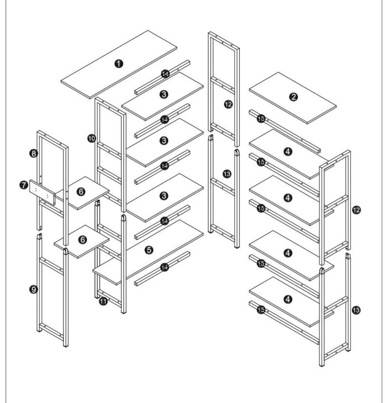
Do not fully tighten all bolts until all parts are in place. Failure to follow these instructions may cause the bolt to misalign during assembly.
