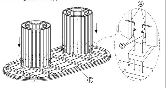
STEP 6: Place the assembled table upright on a level surface. Ensure all table legs are aligned & level, then fully tighten all bolts & screw using allen key (4).
