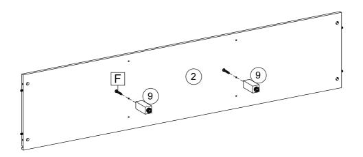
Attach Leg (9) to Bottom panel (2) using 2 x Screw (F).
