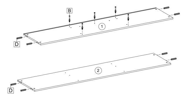
Screw 5 x Cam Bolts (B) into Top Panel (1).
