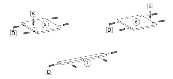
Screw 2 x Cam Bolts (B) into Divider Left Panel (5) and Divider Right Panel (6). Insert 12 x Plastic Dowel (D) into Divider Left Panel (5), Divider Right Panel (6) and Support Panel (7), If necessary, gently tap the Plastic dowels with a mallet.
