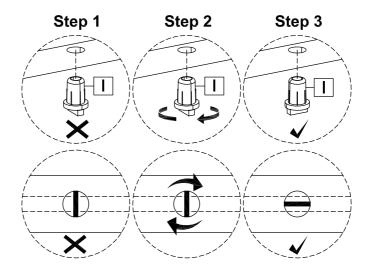
Insert 4 x Bottom Door Pin (I) into Left Door (11) and Right Door (12), Insert 4 x Top Door Pin (J) into Left Door (11) and Right Door (12), Insert 2 x Pin (H) into Left Door (11) and Right Door (12). Turn flat head on Bottom Door Pin until line up with the door as shown.
