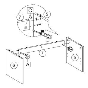
Attach Divider Left Panel (5) and Divider Right Panel (6) to Support Panel (7) using 2 x Cam lock (A), Use a screwdriver to turn the Cam lock clockwise to lock. Paste 2 x Cam Sticker (C) as shown.
