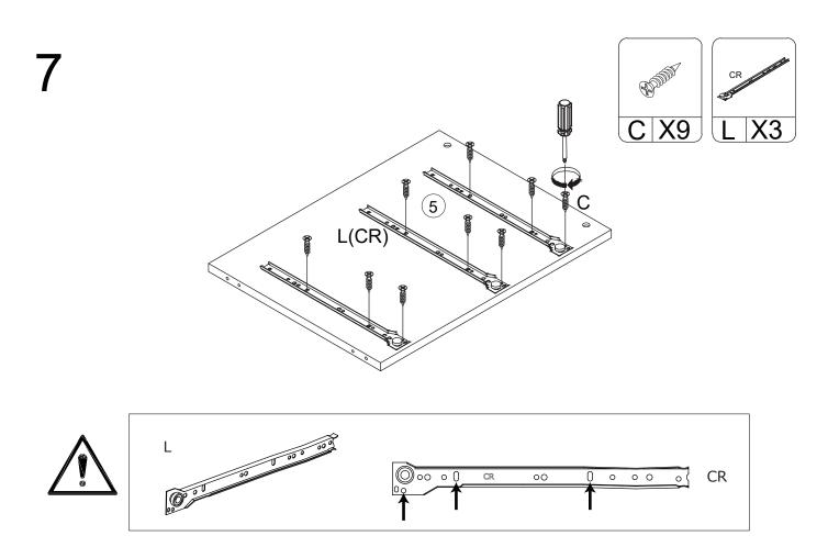
Fix 3 x Slide Tracks L (CR) onto Divider (5) with 9 x Screws (C) using a screwdriver.
