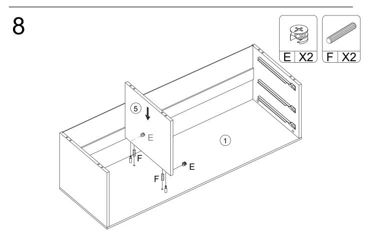
Insert 2 x Dowels (F) into Divider (5) as shown. Position Divider (5) onto the Top panel (1). Insert 2 x Cam nuts (E) into Divider as shown. Use a screwdriver to turn Cam nuts (E) clockwise to lock.
