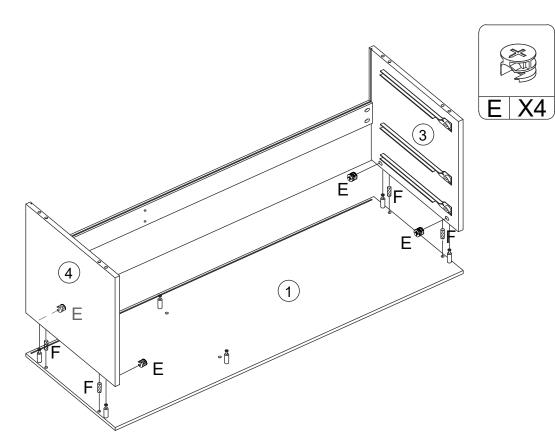
Insert 4 x Dowels (F) into Left side panel (3) and Right side panel (4) as shown. Position the Side panels onto the Top panel (1). Insert 4 x Cam nuts (E) into Side panels (3) and (4) as shown. Use a screwdriver to turn Cam nuts (E) clockwise to lock.
