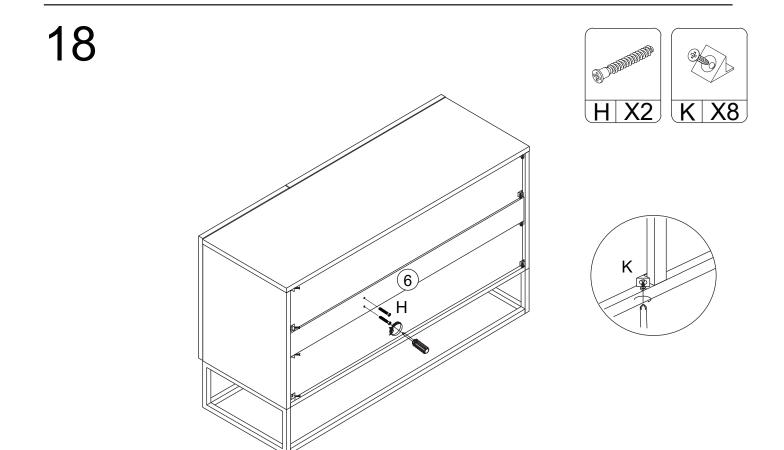
Fix Back support panel (6) to Divider (5) with 2 x Screws (H) using a screwdriver. Fix 8 x Back panel holders (K) to assembled unit with 8 x Screws using a screwdriver.
