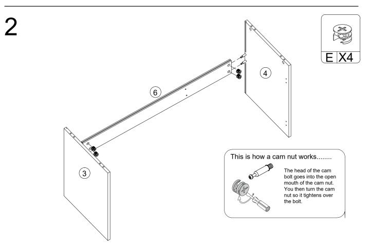
Position Back support panel between Left side panel (3) and Right side panel (4) as shown. Insert 4 x Cam nuts (E) into Back support panel as shown. Use a screwdriver to turn Cam nuts (E) clockwise to lock.
