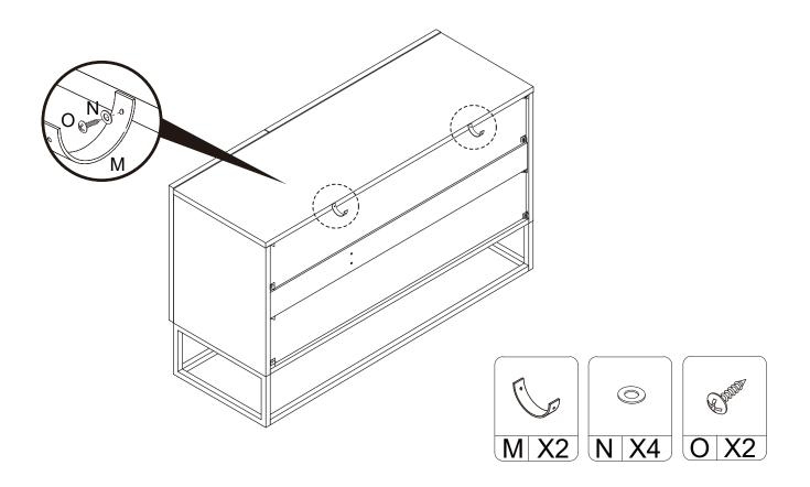
Fix the 2 x Wall straps (M) with 2 x Screws (O) and 2 x Washers (N) to the backside of Top panel as shown. Move the Sideboard into position against a wall.
