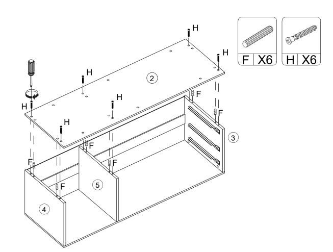
Insert 6 x Dowels (F) into Left side panel (3), Right side panel (4) and Divider (5) as shown. Attach Bottom panel (2) to the assembled frame with 6 x Screws (H) using a screwdriver.
