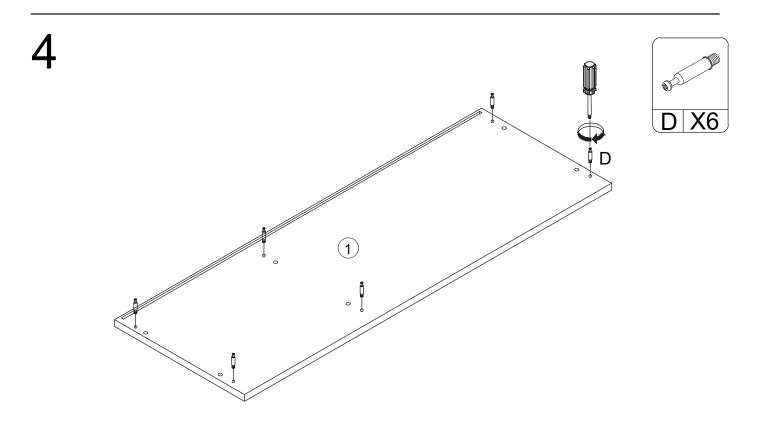
Screw 6 x Cam bolts (D) into Top panel (1) using a screwdriver.
