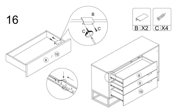
Attach 2 x Handles (B) to Drawer fronts (9) and (10) with 4 x Bolts (C) using a screwdriver as shown. Slide drawer with Drawer Front (8) onto the top two slide tracks as shown. Slide drawer with Drawer Front (9) onto the middle two slide tracks as shown.
