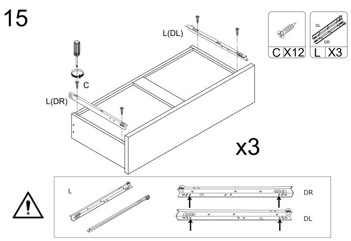
Fix Slider runner L (DL) onto the Left drawer sides with 2 x Screws (C) using a screwdriver. Fix Slider runner L (DR) onto the Right drawer sides with 2 x Screws (C) using a screwdriver as shown. Repeat with the remaining Drawers.
