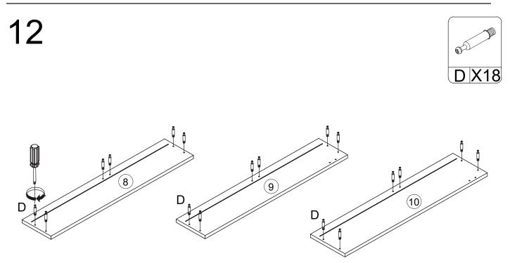
Screw 18 x Cam bolts (D) into Drawer fronts (8), (9) and (10) using a screwdriver as shown.
