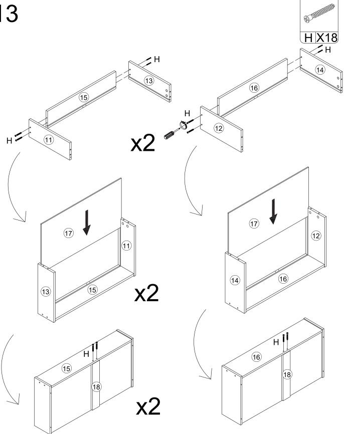
Fix Drawer back panel (15) onto Left drawer side (11) and Right drawer side (13) with 4 x Screws (H) using a screwdriver. Slide Drawer bottom (17) into the grooves of Left drawer side (11), Right drawer side (13) and Drawer back (15) as shown. Fix Drawer bottom support slat (18) onto Drawer back (15) with 2 x Screws (H) using a screwdriver. Repeat with the remaining Drawer panels.
