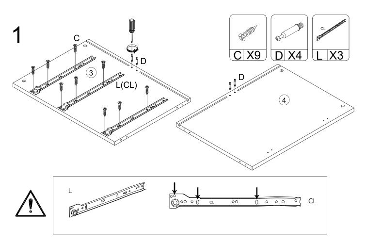
Fix 3 x Slide Tracks L (CL) onto Left side panel (3) with 9 x Screws (C) using a screwdriver. Screw 2 x Cam bolts (D) into Left side panel (3) using a screwdriver. Screw 2 x Cam bolts (D) into Right side panel (4) using a screwdriver.
