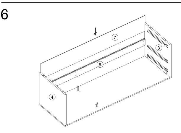
Insert Back panel (7) into the grooves of Left side panel (3), Right side panel (4) and Back support panel (6).
