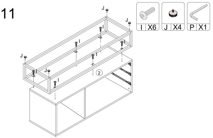
Attach the assembled metal base frame onto the assembled cabinet with 6 x Bolts (I) with Allen key (P). Screw 4 x Adjustable Feet (J) into the metal base frame as shown. With help, turn the assembled unit upright.
