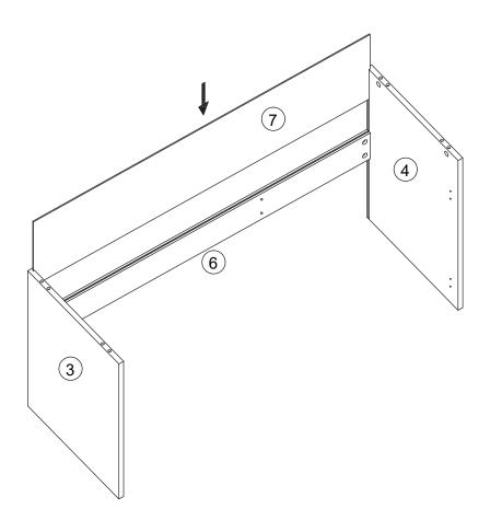
Insert Back panel (7) into the grooves of Left side panel (3), Right side panel (4) and Back support panel (6).
