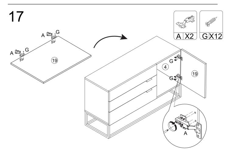
Attach 2x Hinges (A) to Door (19) with 4x Screws (G) using a screwdriver. Attach Door (19) to Right side panel (4) with 8 x Screws (G) using a screwdriver as shown. If necessary, adjust the Hinges (A) using a Screwdriver.
