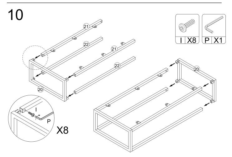
Fix 2 x Metal support rails (21) and 2 x Metal support rails (22) between 2 x Metal leg frames (20) with 8 x Bolts (G) using Allen key (N) as shown.
