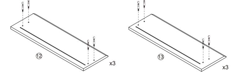
Attach 8 x Cam Bolts (C) to Drawer Fronts (12 & 13) as shown. Tighten with a Phillips Head Screwdriver.
