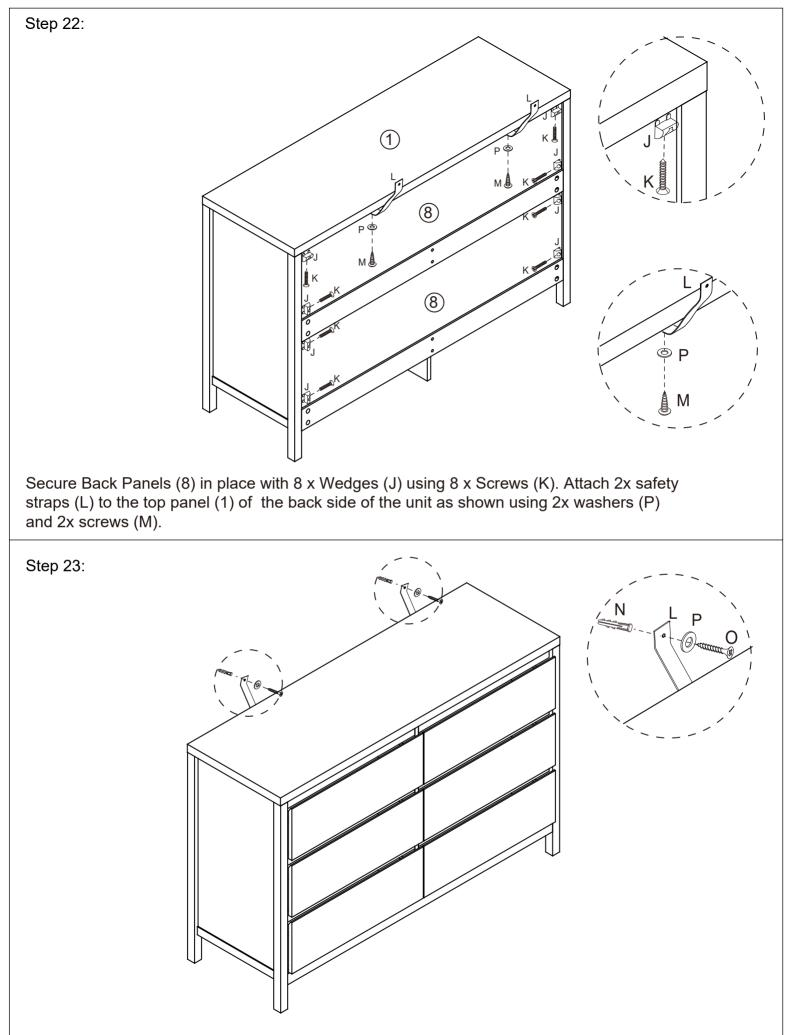
Move the unit to the final position, and attach the safety strap to the wall securely. Make sure it is firmly attached and snug fit. If you are unsure, please seek professional advice on how to attach this safety strap to your specific wall.
