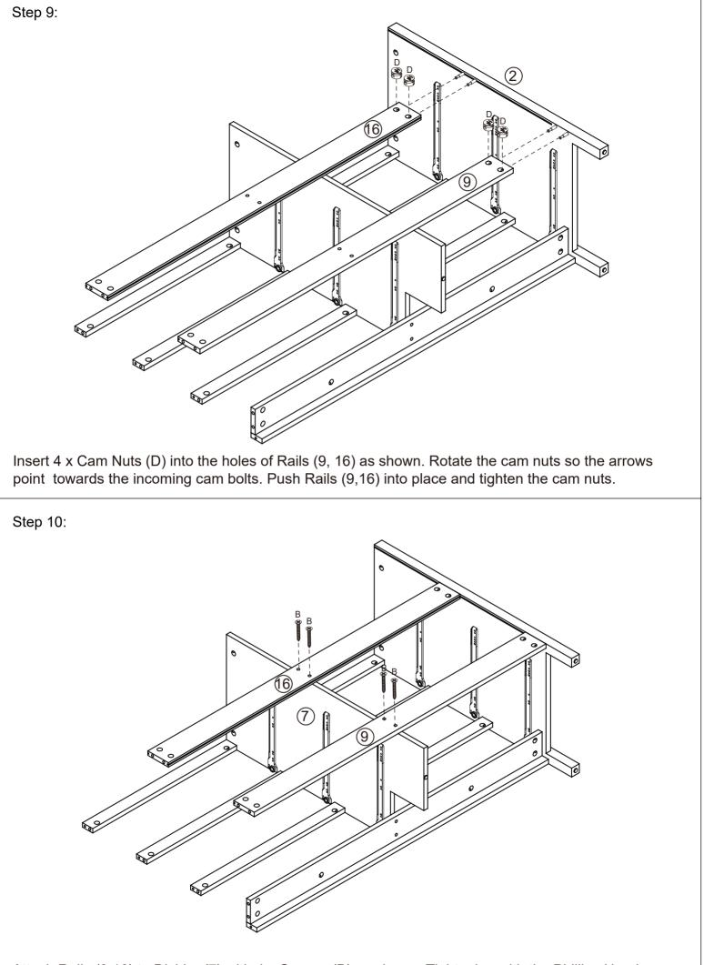
Attach Rails (9,16) to Divider (7) with 4 x Screws (B) as shwon. Tightening with the Phillips Head Screwdriver.
