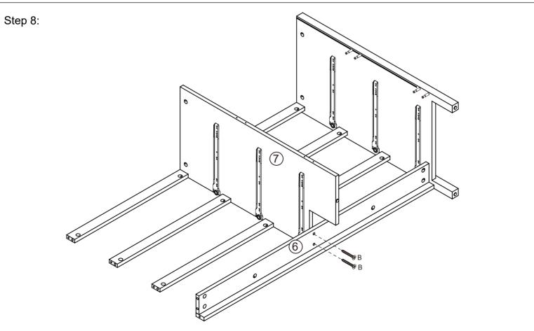
Attach Rail (6) to Divider (7) with 2 x Screws (B) as shwon. Tightening with the Phillips Head Screwdriver.
