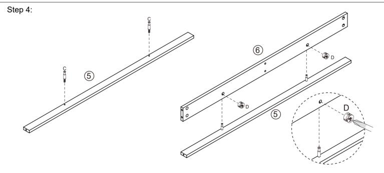
Attach 2 x Cam Bolts (C) to Rail (5) as shown. Tighten with a Phillips Head Screwdriver. Insert 2 x Cam Nuts (D) into the holes of Rail (6). Rotate the cam nuts so the arrows point towards the incoming cam bolts. Push Rail (5) into place and tighten the cam nuts.
