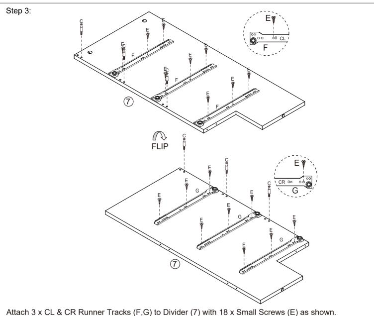
Tighten with a Phillips Head Screwdriver. Attach 6 x Cam Bolts (C) to Divider (7) as shown. Tighten with a Phillips Head Screwdriver.
