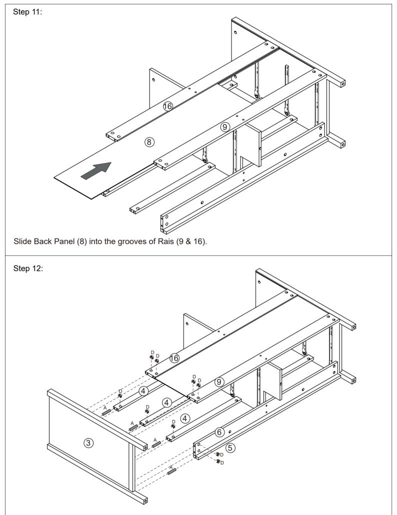
Insert 4 x Dowels (A) into Right Side Panel (3) as shwon. Insert 9 x Cam Nuts (D) into the holes of Rails (4, 6, 9, 16). Rotate the cam nuts so the arrows point towards the incoming cam bolts. Push Right Side Panel (3) into place and tighten the cam nuts.
