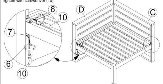
**STEP 6:** Place the assembled chair upright on a level surface. Ensure all chair legs are aligned & level, then fully tighten all bolts & screw using allen key (7). Your chair is now ready for use.
