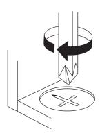
Tum cam lock clockwise to tighten.
