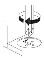
Turn cam lock clockwise to tighten.
