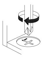
Turn cam lock clockwise to tighten.
