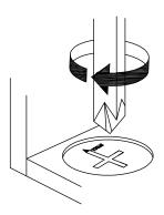
Turn cam lock clockwise to tighten.
