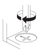
Turn cam lock clockwise to tighten.
