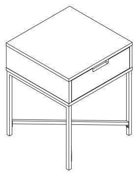
Maximum recommended weight is 10kg on top and 5kg for the drawer.
