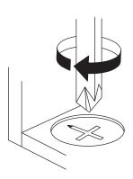
Turn cam lock clockwise to tighten.
