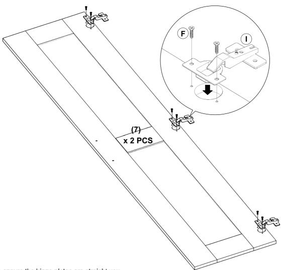
TIP: To ensure the hinge plates are straight you could use the straight edge of another panel and place on top and position the edge against the hinge plates, ensure the panel is aligned properly with the door panel and double check all hinges are nice and straight before you tighten / secure the hinges onto the panel.
