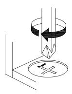
Turn cam lock clockwise to tighten.
