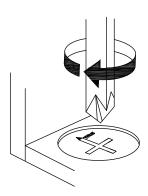
Turn cam lock clockwise to tighten.
