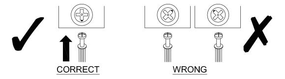
When fitting cam lock, ensure starting position is correct before you insert connecting quickfit.
