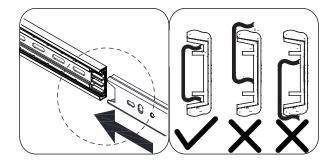
• Insert the drawer into the assembled frame as show below. Keep each side of the drawer straight and aligned correctly to the sliders on the assembled frame.
