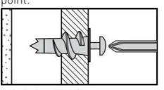
**2. Plasterboard Wall Plug** For use when attaching light loads onto plasterboard partitions.
