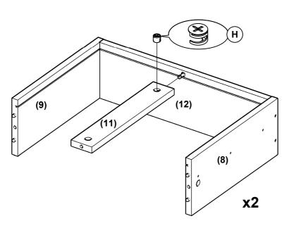
Note: Its important not to over-tighten screws on the drawer sides until all sides are aligned and the drawer base is inserted. Always keep drawer flat in this step so the groove for the base will align correctly
