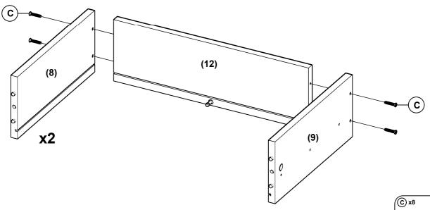
**Note:** Its important not to over-tighten screws on the drawer sides until all sides are aligned and the drawer base is inserted. Always keep drawer flat in this step so the groove for the base will align correctly.
