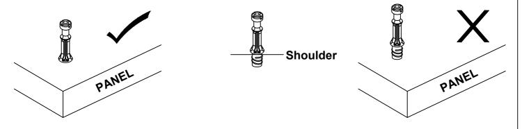
Tighten quickfit until shoulder is flush with panel . Do not overtighten or undertighten.
