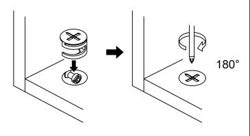
Turn cam lock clockwise to tighten.
