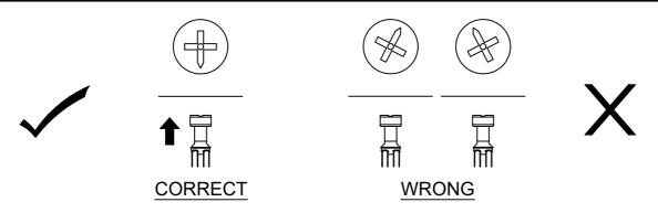
When fitting cam lock, ensure starting position is correct before you insert connecting quickfit.
