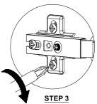
After adjust, tighten the screw.
