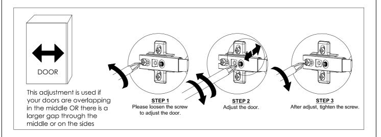
Follow the adjustments and make sure the middle pin is correctly installed as per previous instructions. If the middle pin isn't correctly installed then this adjustment will not work correctly.
