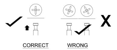
When fitting cam lock, ensure starting position is correct before you insert connecting quickfit.
