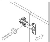
**A.** Lateral adjustment by screw adjusting
