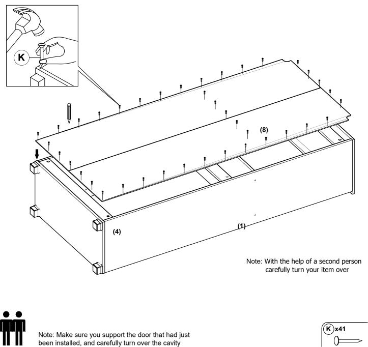
ready to attach the backing board in the next step.
