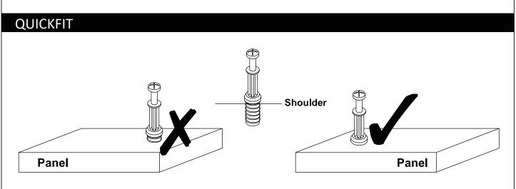
Tighten quickfit until shoulder is flush with panel. Do not overtighten or undertighten.
