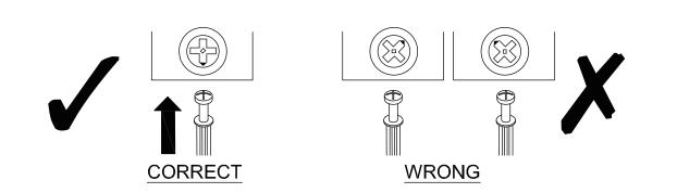
When fitting cam lock, ensure starting position is correct before you insert connecting quickfit.
