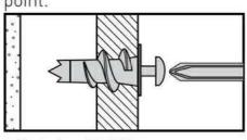
2. Plasterboard Wall Plug For use when attaching light loads onto plasterboard partitions.
