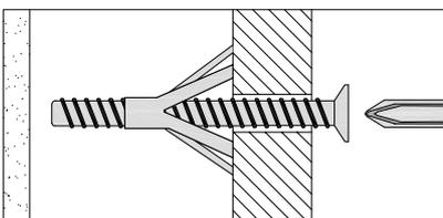
For use with plasterboard partitions or hollow wooden doors.
