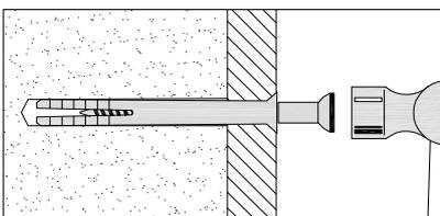
For use with walls stuck with plasterboard. The hammer fixing allows it to be fixed to the wall rather than the plasterboard. Always check the fixing is secure to the retaining wall.
