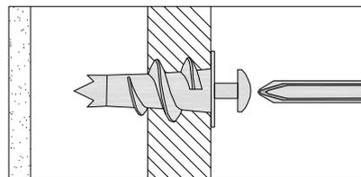
For use when attaching light loads on to plasterboard partitions or hollow wooden doors.
