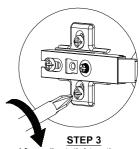
After adjust, tighten the screw.
