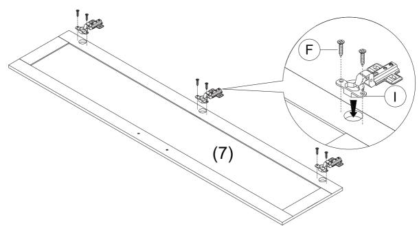
**TIP:** To ensure the hinge plates are straight you could use the straight edge of another panel and place on top and position the edge against the hinge plates, ensure the panel is aligned properly with the door panel and double check all hinges are nice and straight before you tighten / secure the hinges onto the panel.
