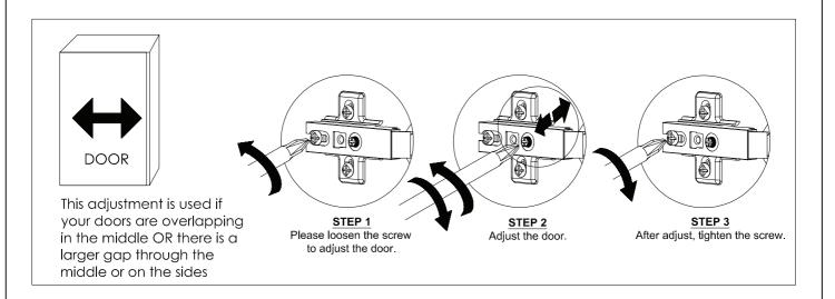
Follow the adjustments and make sure the middle pin is correctly installed as per previous instructions. If the middle pin isn't correctly installed then this adjustment will not work correctly.
