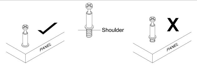
Tighten quickfit until shoulder is flush with panel. Do not overtighten or undertighten.
