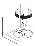
Turn cam lock clockwise to tighten.
