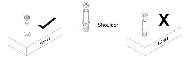
Tighten quickfit until shoulder is flush with panel. Do not overtighten or undertighten.
