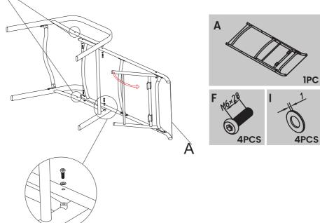
4.2 ★ Please assemble this screw first, so that the next 3 screws will be very easy to tighten.
