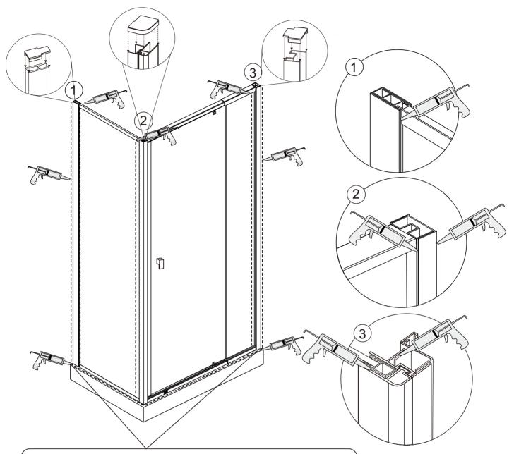
Do not silicone floor section from inside to allow moister and condensation to drain back into the shower.
